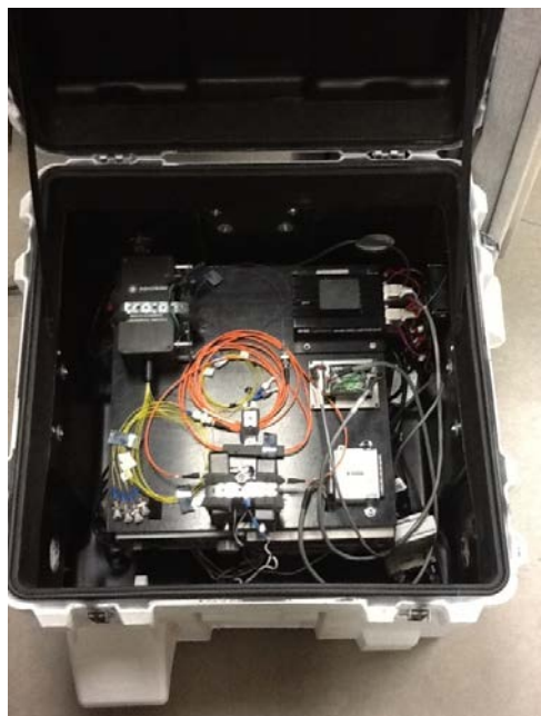
Electronics and optics packaged in a weatherproof enclosure for field studies.
